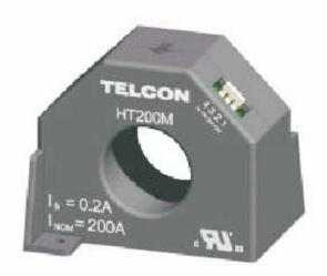
The HT200M is a closed loop Hall Effect Current Transformer which is suitable for Panel Mounting. Provision is made for the primary conductor to be threaded through a single hole. Rated for 200A continuous operation, it offers high accuracy and bandwidth and high electrical isolation. The unit is UL listed, File No. E198118.
