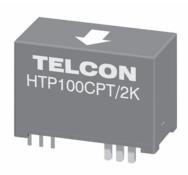
The HTP100CPT/2K is a closed loop Hall Effect Current Transformer suitable for measuring currents up to 100A. The product provides an output current into an external load resistance which is galvanically isolated from the primary conductor. All contacts, including the primary, are designed for PCB mounting.
