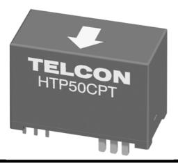
The HTP50CPT is a closed loop Hall Effect Current Transformer suitable for measuring currents up to 50A. The product provides an output current into an external load resistance which is galvanically isolated from the primary conductor. All contacts, including the primary, are designed for PCB mounting.
