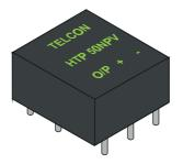
The HTP50NPV is a compact, multiple primary turn closed loop Hall Effect Current Transformer suitable for measuring currents up to 50A. It is designed for those applications where connection to the primary circuit is made directly on the printed circuit board
